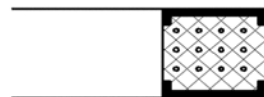
TREGRAPH ® AR ring, reinforced with nickel alloy wire and both sides sheets of AISI 316
