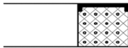
TREGRAPH ® AR ring, reinforced with nickel alloy wire and one-side sheet of AISI 316
