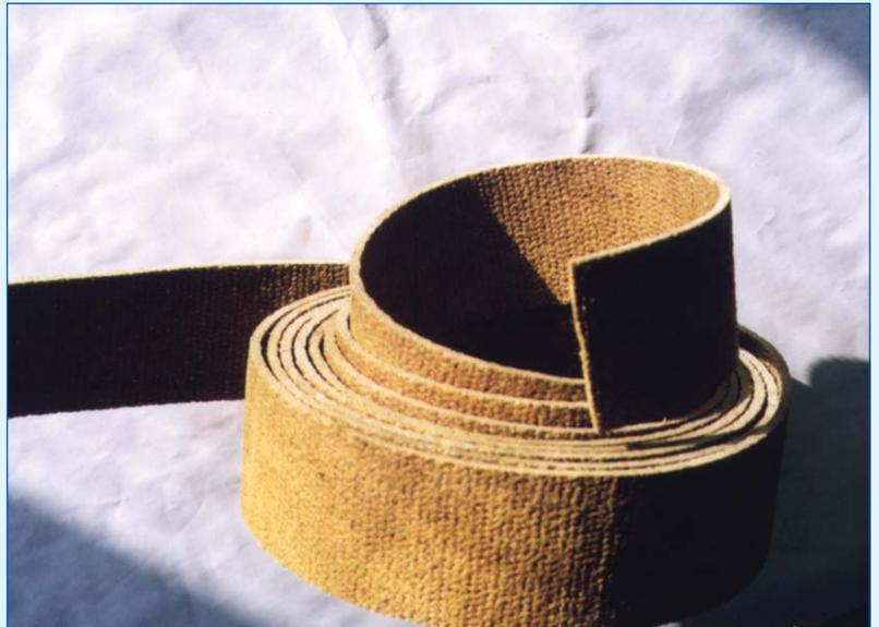
Reinforcement is made with soft copper/brass wire, which improve strength and work of the friction product, through transferring of the heat from the contact zone and stabilize stopping process, especially in the cases of low speed of slipping.
